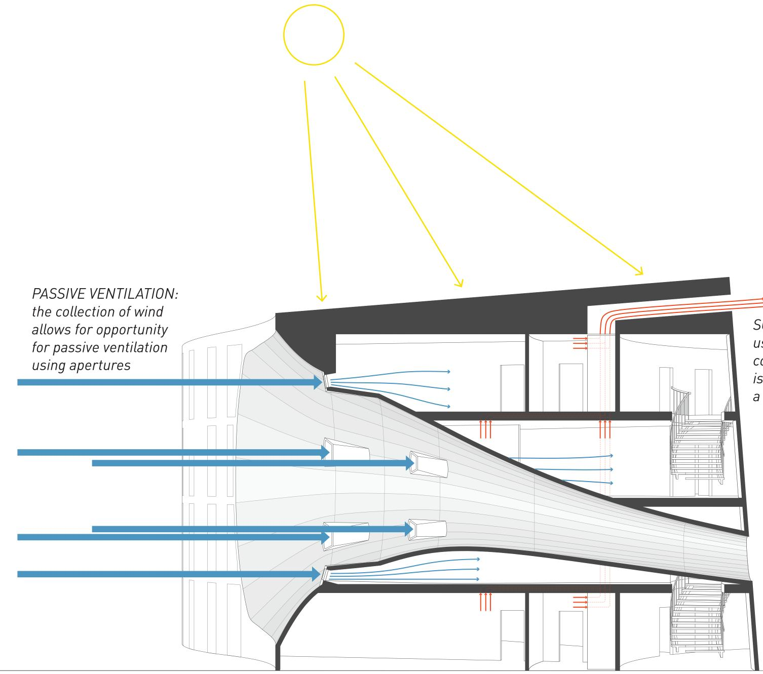
SOLAR CHIMNEY: using heat and convection, warm air is exhausted through a roof opening.
